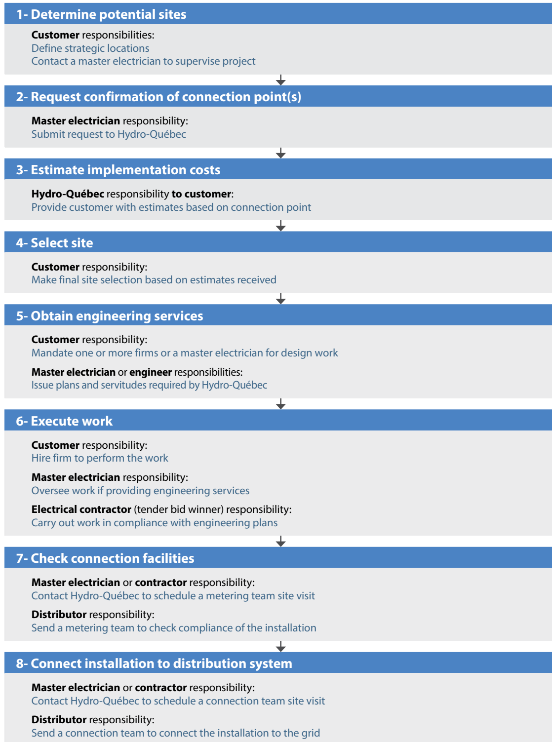
Figure 16 – Flowchart for installing charging stations
