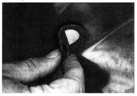
A grommet made from VW fuel line.
