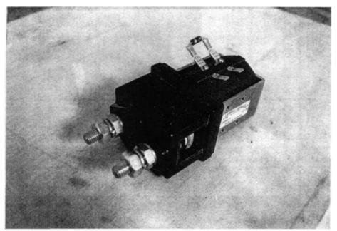
A main contactor, with a diode to suppress voltage spikes.
