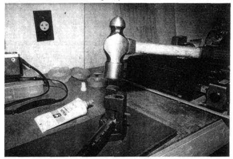
Crimping lugs with a cradleand-punch style tool. The entire crimping sequence is as follows: First, use a box razor knife to strip 5/8" of insulation from the end of the cable. Be careful not to cut the copper strands inside.
