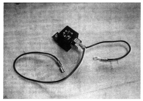
A wiring loom tap connected to the keyswitch relay.
