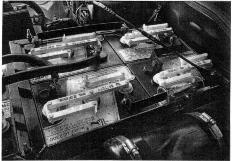
A battery pack using copper strap interconnects. Note fusible link in one interconnect. Drill 5/16" holes in the strap ends and deburr them before bending the straps. Also, slide the shrink tube onto the strap before bending it, then shrink it into place afterwards.
