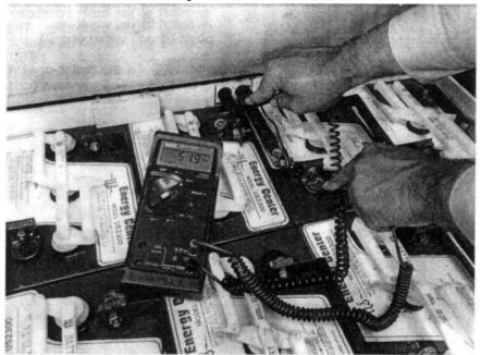
Checking battery pack voltage with a voltmeter.
