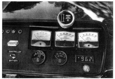
An LED bar gauge (top), panel meters (center), round automotive-style gauges (bottom left), and a digital gauge (bottom right). Note how the face on the leftmost panel meter is faded from the sun. For these reasons, I prefer standard automotivestyle (and quality) round analog gauges. I find them to be accurate, readable, durable, and attractive.
