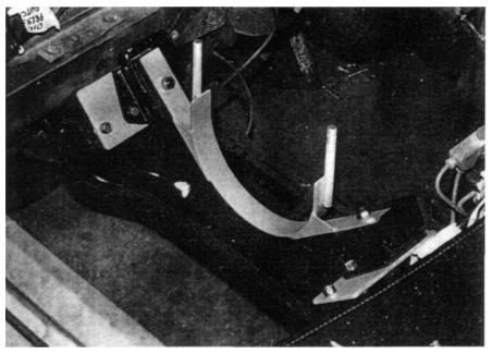
A cradle-type mount, mounted to original (black) motor mounts, and (grey) setback plates. For a transverse engine car, use a plate mounted to the anti-drive end of the motor and extending into a mounting bracket.
