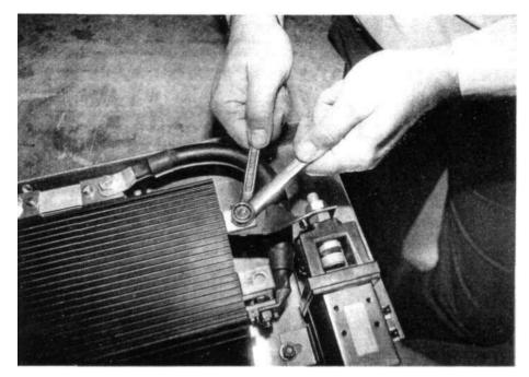
Use two wrenches when fastening lugs to controller terminals.
