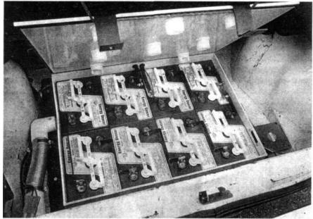
Rear Voltsrabbit<sup>™</sup> battery box, with ventilating fan at lower right and exhaust duct at left. Note holddown blocks welded to inside of lid. PVC fittings can be very useful for ventilation ducting. Elbows of various diameters and degrees of bend are available, as well as adaptors to fit round hoses to square holes. Aluminum Volkswagen accordion hose and clothes drier hose are both useful options.
