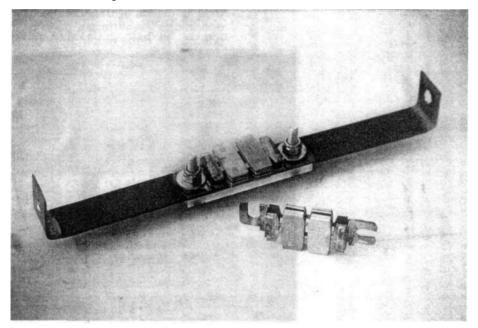
A bare fusible link, and one mounted on a plexiglass block in a battery interconnect.
