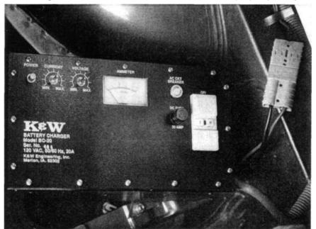
An onboard charger connected by an Anderson connector.
