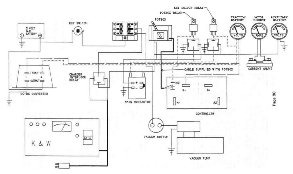
inline fuses, but the same thing can be done better by using a fuse block instead of an ordinary terminal block. I prefer the type with spade-style fuses. Use fuses rated at double the amperage of the component.
