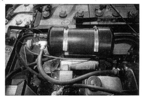
A power brake vacuum system, including pump, reservoir, switch, and brass fittings.
