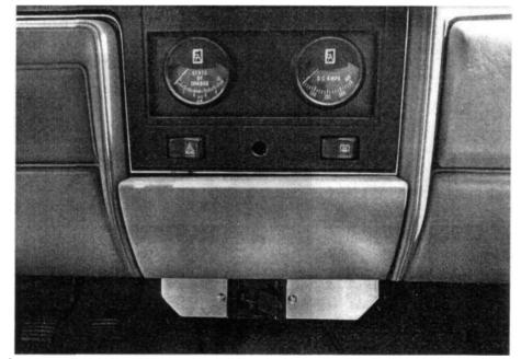
The dash of a late model Voltsrabbit<sup>™</sup>, showing an ammeter and state-of-charge gauge, and the circuit breaker at the bottom.
