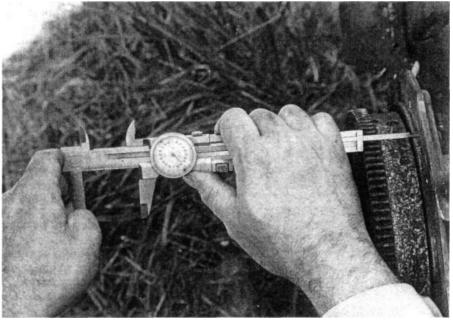
The 'magic number' is the distance between the rearmost surface of the engine and the rearmost flat surface of the flywheel.
