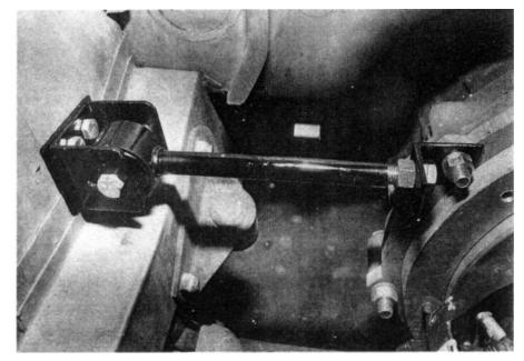
Install the torque rod between the chassis and the
