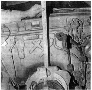
Measure the distance from the top of the transmission bell housing to some stationary mark. (It's easier to see in this photo, with the electric motor already in place, than in the original car with the gas engine.) This measurement will help you reinstall the transmission with the electric motor in exactly the same position. This is important for such things as driveshaft angularity and shift linkages.
