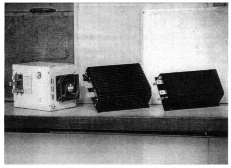
PMC controller evolution: the early model DCC 96, the long-popular model 21, and the current MOSFET model 1221.
