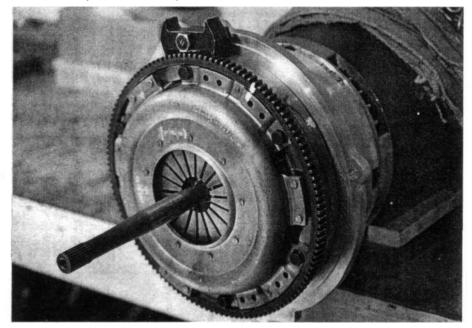
Clutch parts being mounted on the motor and adaptor. (Note flywheel lock tool at top, and paint mark for aligning flywheel and pressure plate.) The flywheel is part of the clutch assembly. When you are installing the adaptor, this is the time to replace the clutch pressure plate, disc, and release bearing with new parts. If you do it right the first time, you won't have to change the clutch again until you replace the motor brushes at 80,000 miles.
