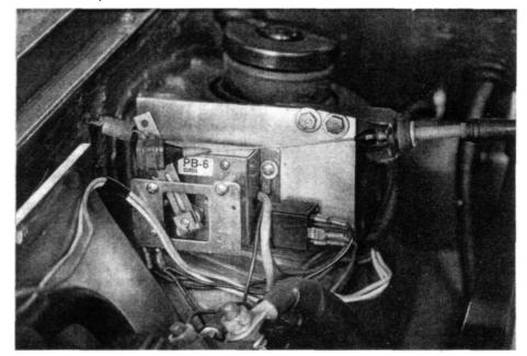
In the Voltsrabbit<sup>TM</sup>, the potbox uses the original cable for the throttle, part of the original bracket for the cable, and an auxiliary throttle return spring.
