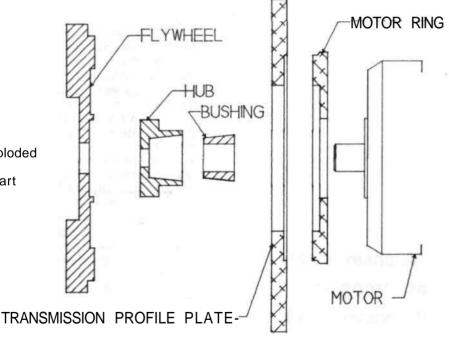
There are two reasons for this design. The first is weight and economy. The minimum thickness needed for the plate is determined by the space needed for the hub. If the profile plate were this thick, it would be very heavy and expensive. The ring, which is the diameter of the motor rather than of the transmission, is much more light and affordable.
