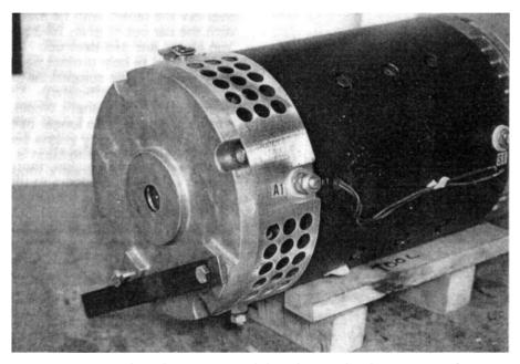
An anti-rotation strap installed on a motor for bench work. Any time you are tightening a circular pattern of bolts, make several passes over the entire sequence, and use a criss-cross pattern. That is, don't try to tighten one bolt all the way, then the one next to it, and so on. This will cause the piece you are installing to tilt slightly, and you will not get a proper tight fit when you are finished. You may even damage threads.
