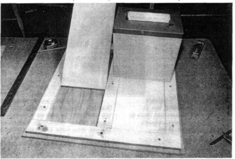
Insulation can be simply a second layer between the box and batteries, or it can be a third layer in the middle of a 'sandwich' box wall or floor. In the two-layer
