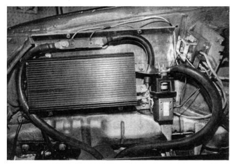
A controller, contactor, and shunt, mounted on an aluminum component board which also serves as a heatsink for the controller.
