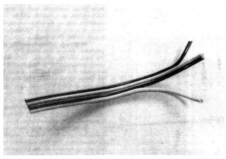
Four-in-one trailer wire makes a tidy ready-made loom.
