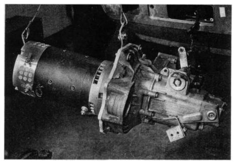
Motor/adaptor/transmission assembly ready to be installed in the car. In order to do this, you will need to design your motor mount precisely. In most air-cooled Volkswagens, no motor mount is necessary. The electric motor hangs off the transmission, just like the original gas engine did. For all other cars, read on.
