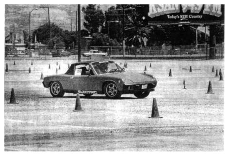
This high-performance electric sports car (a converted 914 Porsche) has a top speed of 90 mph and a range of over 120 miles on a single charge. **Speed.** Most modern EVs can do highway speeds of 50 - 60 mph. A car that is very heavy before conversion will do less well. A very light car such as a kit car, or a very aerodynamic sports car, may have a top speed of 80 - 90 mph. Acceleration is good, and is directly related to the weight of the car and the quality of the components used.
