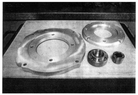
An adaptor, showing the transmission profile plate, the motor ring, the motor shaft bushing, and the hub. There are several styles of adaptor hubs. Most of them are problems waiting for the worst possible time to happen. All the power of that motor passes through this little hub the size of a hockey puck. This, also, is not a place to skimp.
