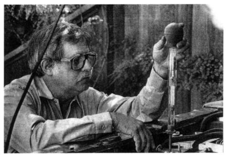
Testing specific gravity with a hydrometer.
