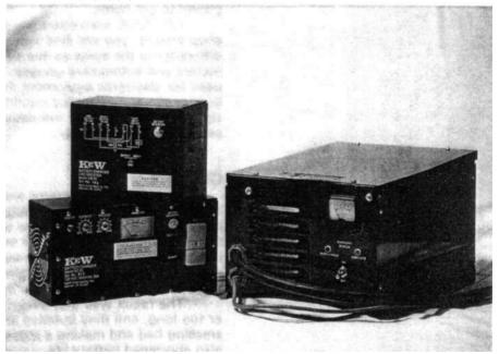
A 110-volt input charger, (bottom left), a booster unit (top left) for charging a pack of 114 volts or more with the 110-volt input charger, and a 220-volt input charger (right). In the past, it has usually been necessary to choose one input voltage or the other. The 110-volt system had a further advantage because it was the first to come out in the smaller, compact version.
