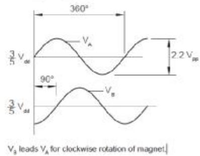
Usually we just need to configure two parameters in user program according to the specification of Sin/Cosin speed sensor. Please click Motor button in the user program.
