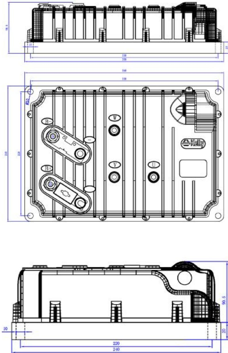
Figure 1:KLS14401-8080/IPS mounting holes' dimensions (dimensions in millimeters)
