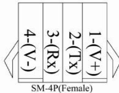
**Figure 9:** SM-4P connector for communication interface on KLS8080I controller
