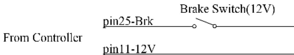
**Figure 6:** Wiring of brake switch(12V): 12V is provided by KLS8080I controller on pin11
