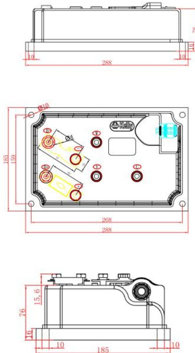
Figure 1:KLS72501-8080/IPS→KLS14301-8080/IPS mounting holes' dimensions (dimensions in millimeters)
