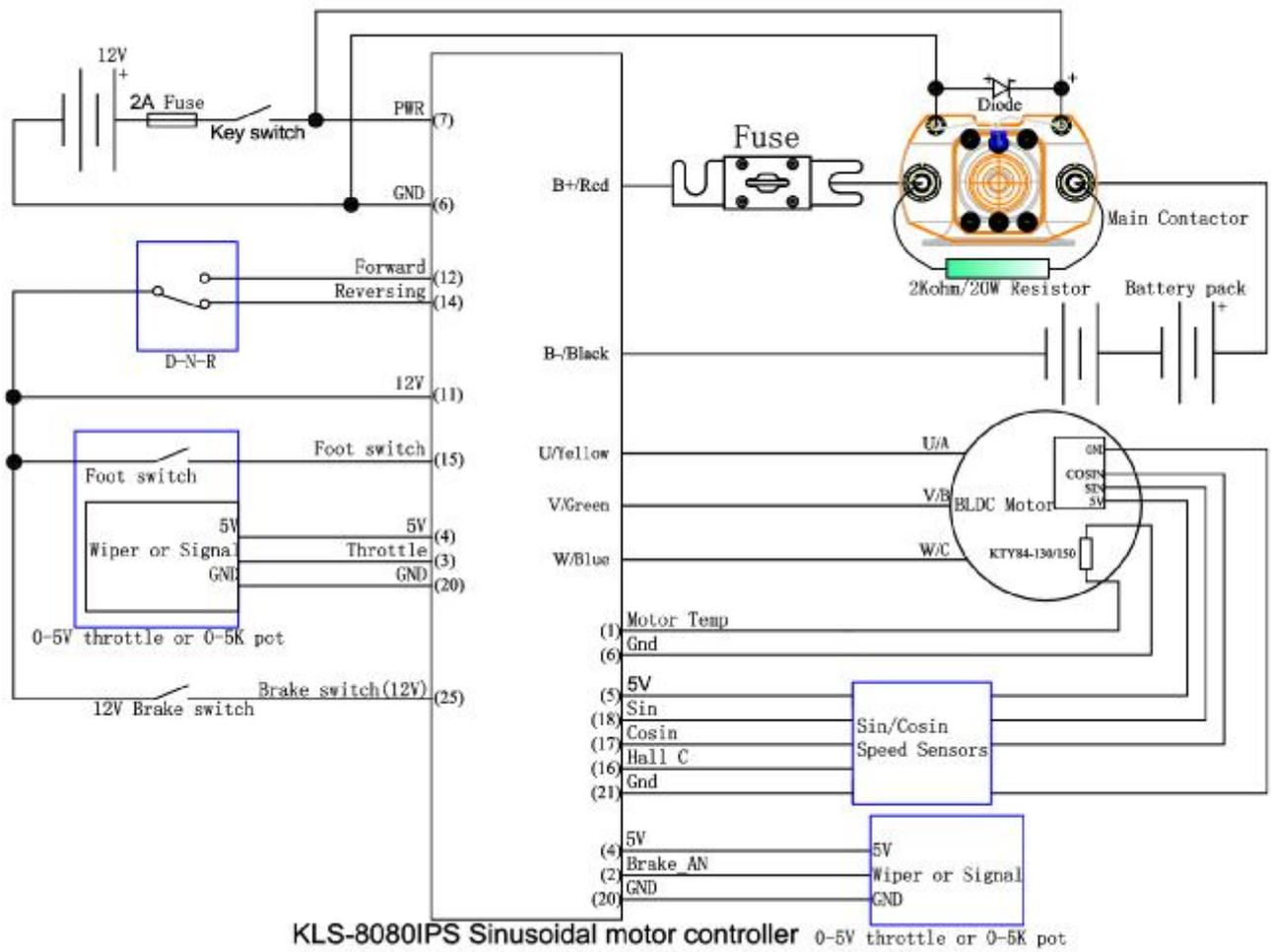
**Figure 4: KLS8080IPS controller standard wiring**
