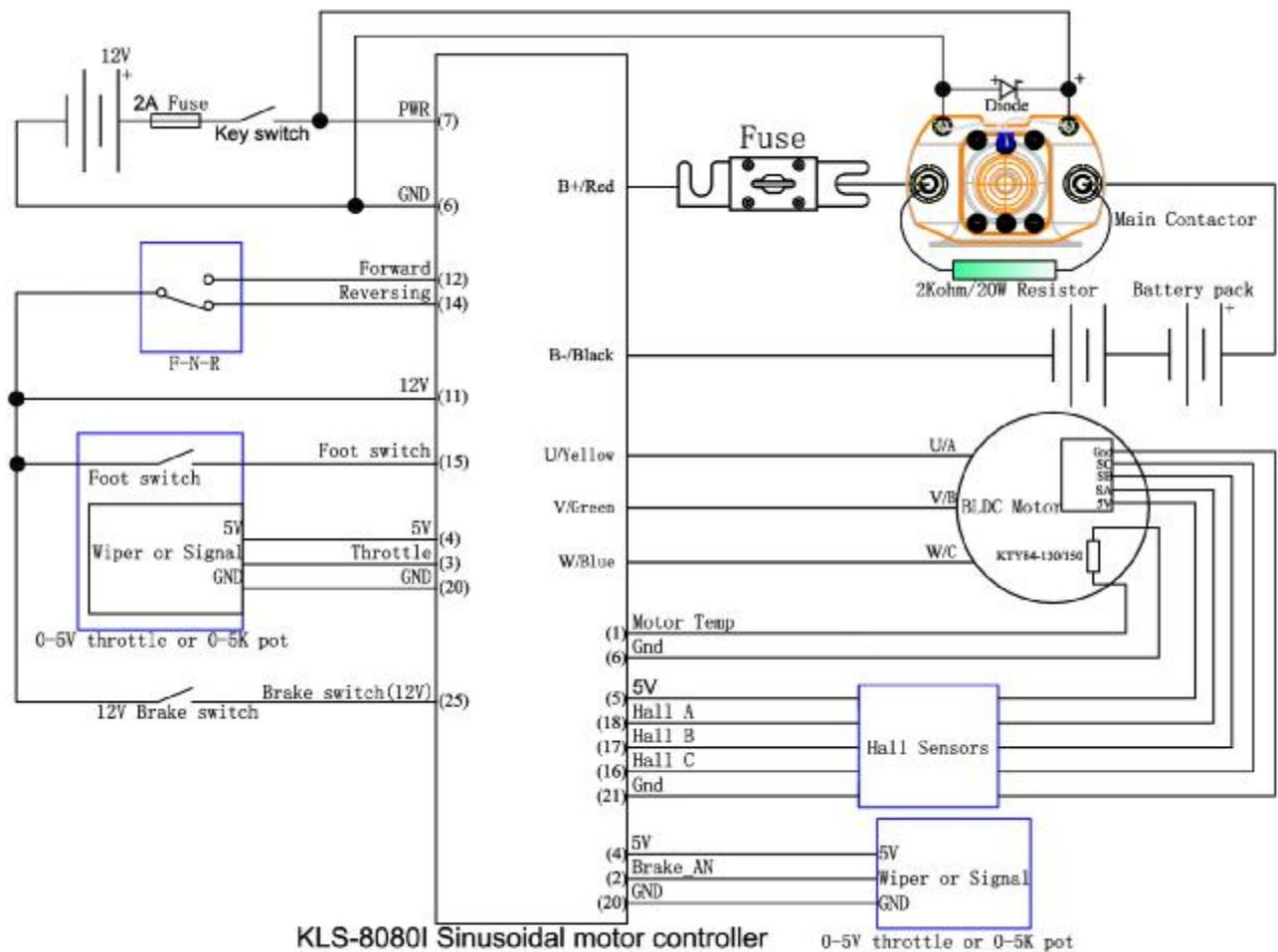
Figure 3: KLS8080I controller standard wiring
