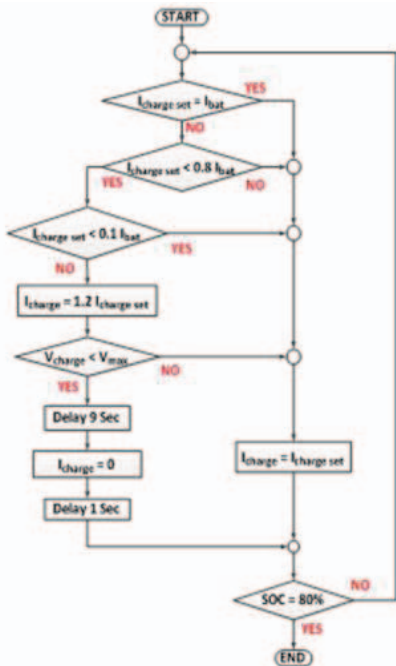
Fig. 6. Flow chart diagram of proposed quick charging technique.
