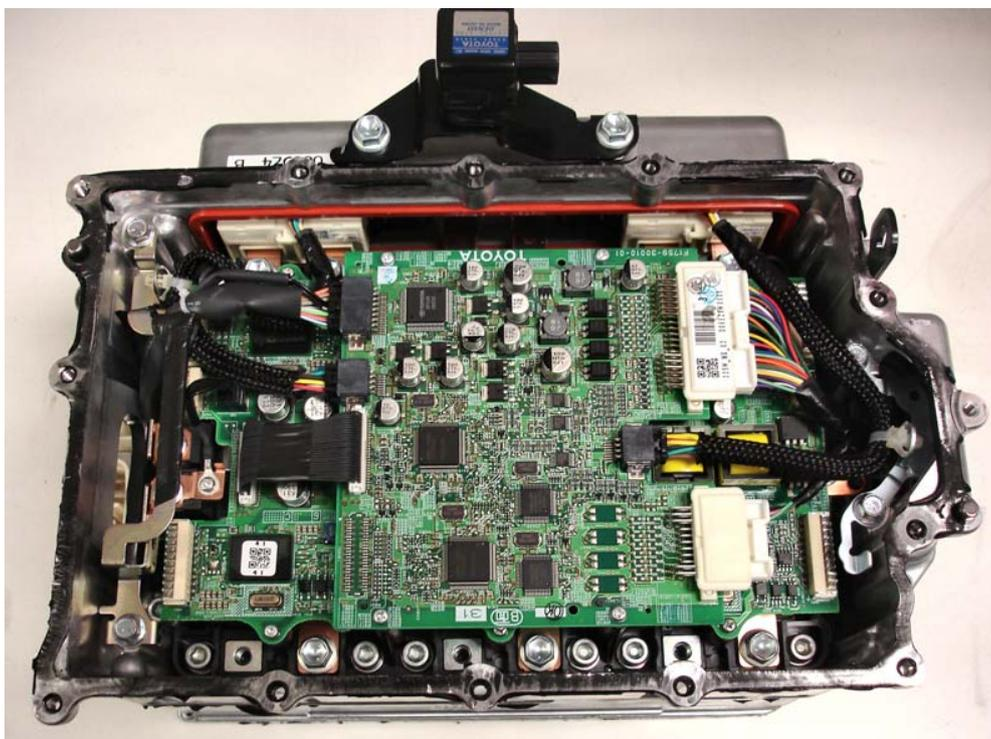
**Fig. 2.4. Inverter compartment (upside down) with dc-link capacitor and casing removed.**
