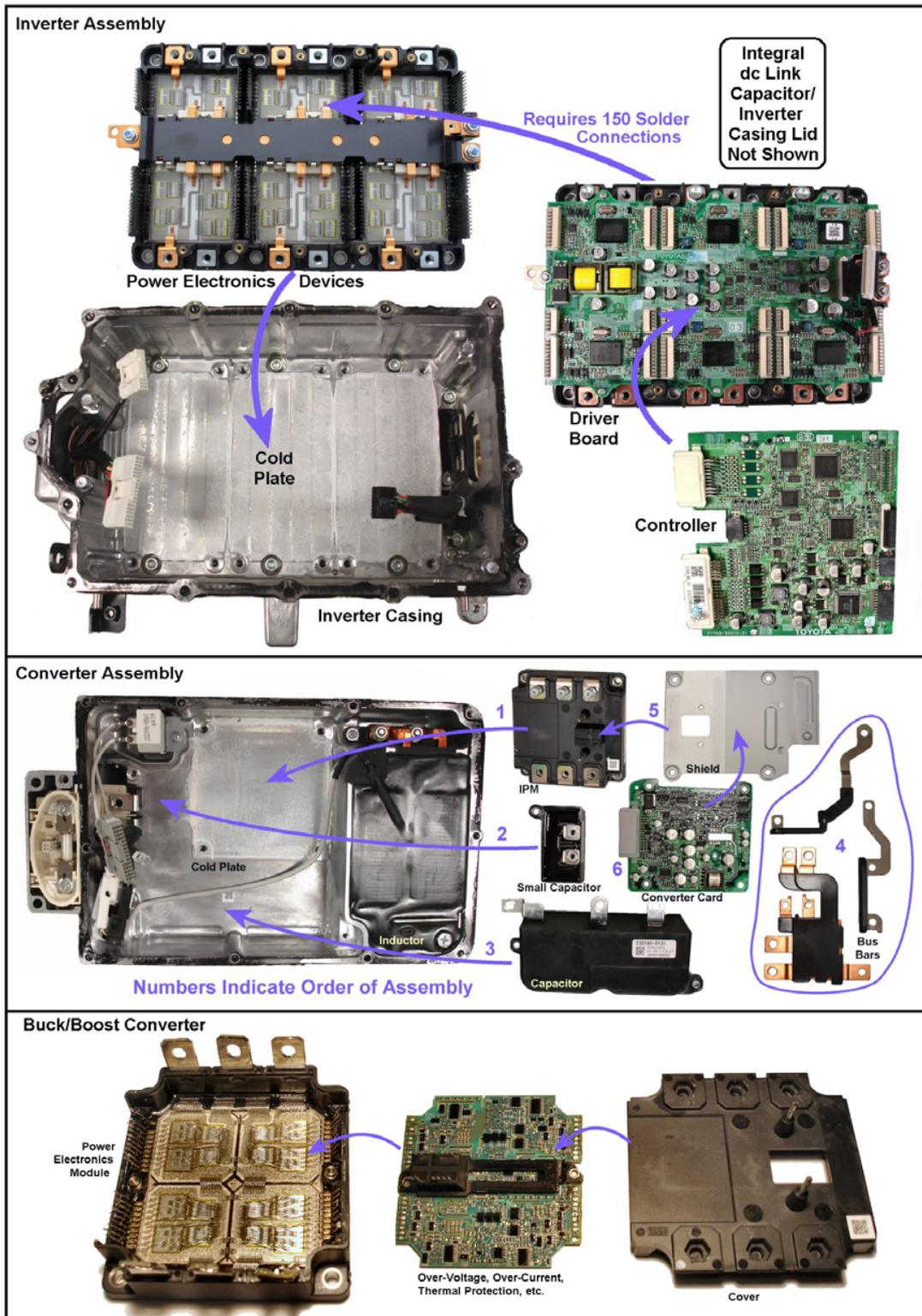
Fig. 2.5. General assembly and packaging of the Camry inverter and converter.
