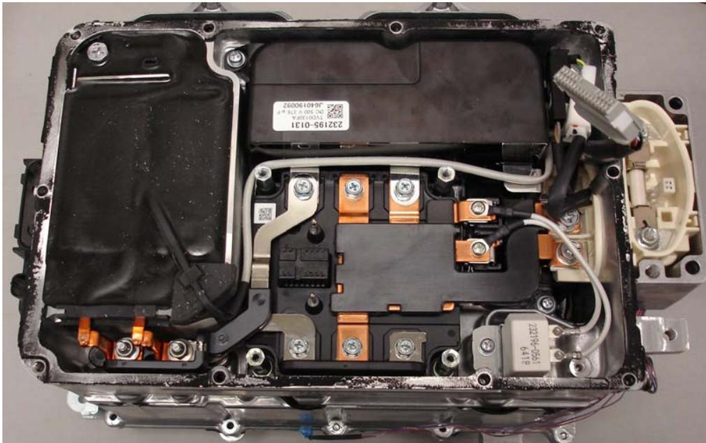
**Fig. 2.3. Boost converter compartment with lid and intelligent power module (IPM) driver board removed.**
