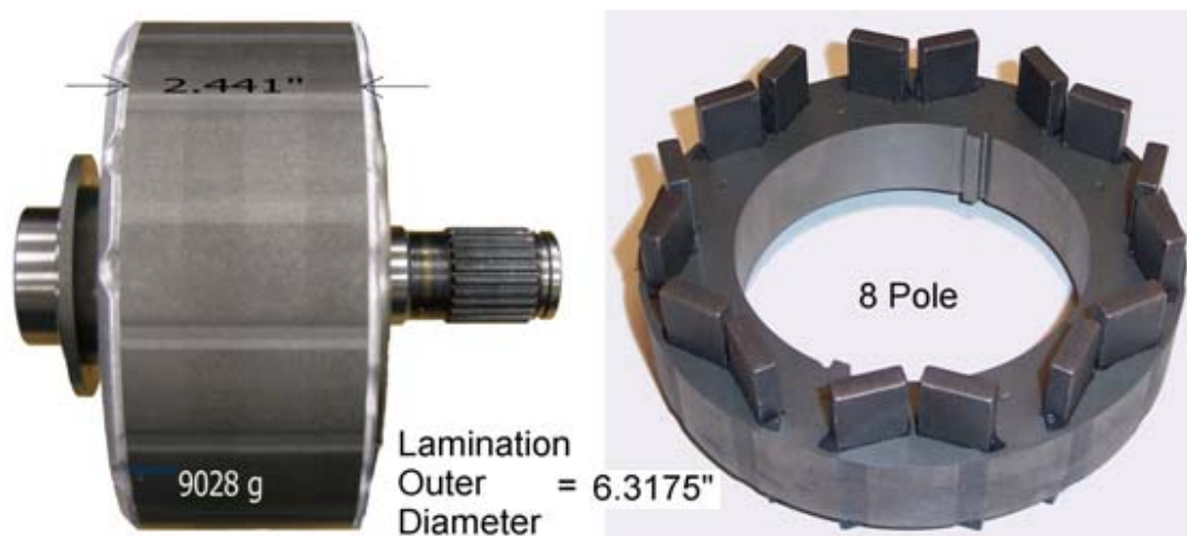
Fig. 2.67. Camry rotor assembled (left) and partially disassembled (right).
