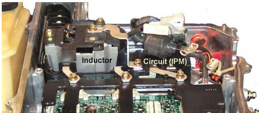
**Fig. 2.8. Non-optimized packaging used in the 2004 Prius converter.**
