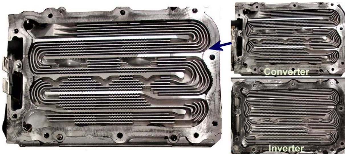
**Fig. 2.6. Coolant flow paths in mating converter and inverter cold plates.**
