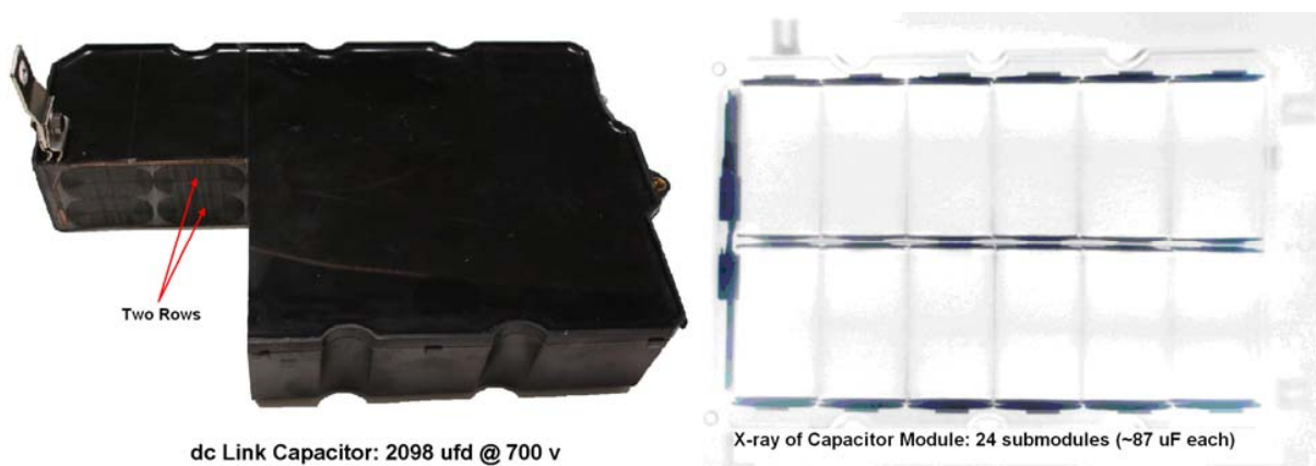
Fig. 2.10. Cutaway of dc-link capacitor removed from shell (left) and x-ray of module (right).
