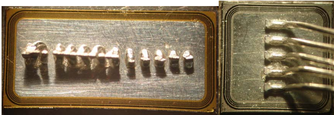
Fig. 2.19. Close-up view of Camry inverter diode (left) and Prius inverter diode (right).
