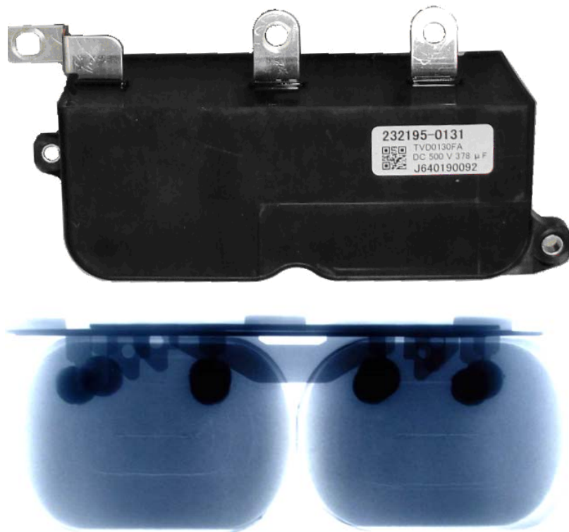
Fig. 2.11. Battery level capacitor (upper) and x-ray of module (lower).
