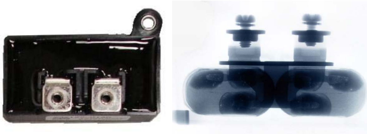
Fig. 2.12. Small dc-link capacitor: overhead view (left) and x-ray of module – side view (lower).
