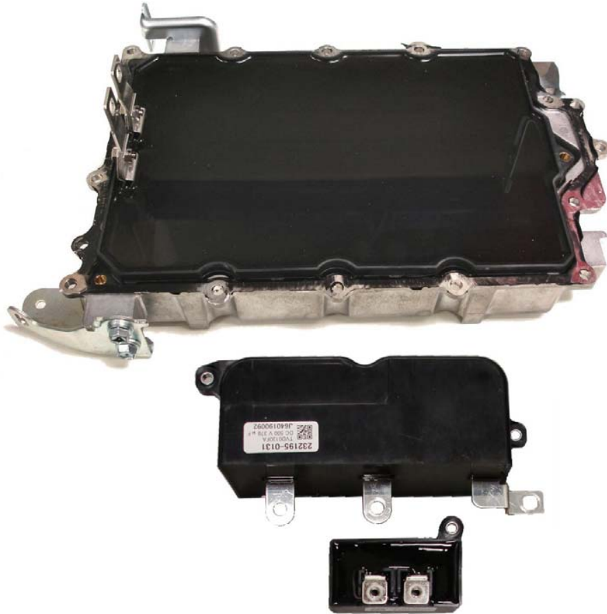
Fig. 2.9. Comparison of all capacitors located within Camry PCU.
